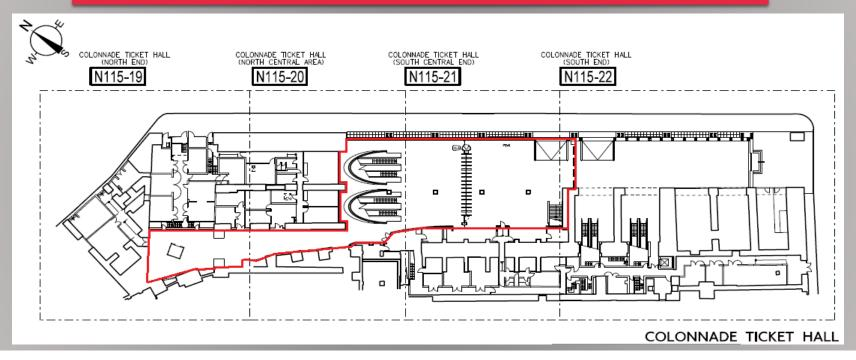
The application area is described by the red line. The lift is situated in the extreme left (NW) of the diagram. The escalators and ticket barriers are in the middle.
